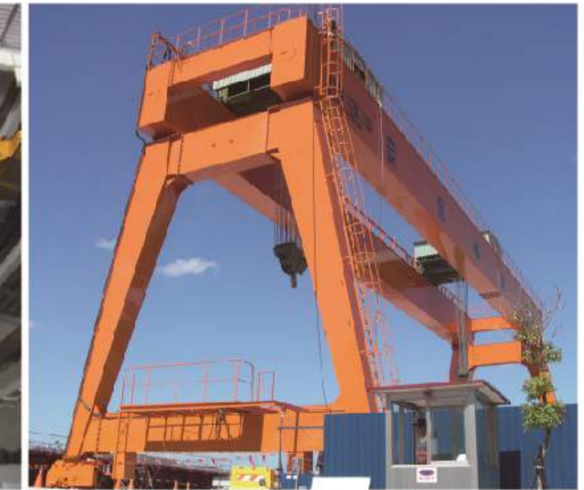
2010 Airport Metro Line 260 Tons Gantry Crane Project
